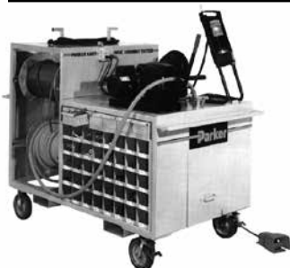
Pictured left is a complete on-site hose assembly workstation, the Parker Kart:
